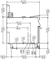
EQ = Equipotential screwG = Gas connection
