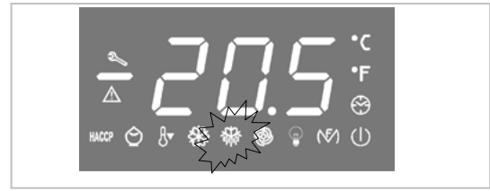
This LED indicates that defrosting is in progress
